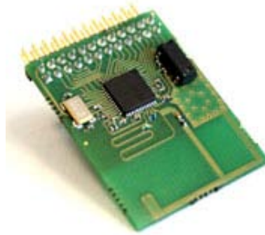
Figure 23: Aurel XTR-ZB1-XLI module Reprinted with permission from Aurel
